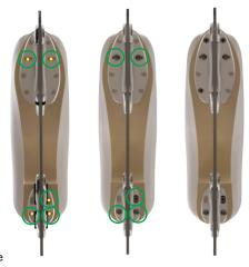
Check the straightness of the blade and make adjustments if necessary.
